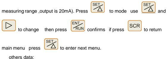
Blanking dist blank mode the min distance from sensor to level that the unit cannot operate.(30cm-60cm)
