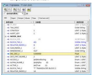
Figure 4.6 Parameter configuration for display block
