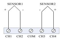
Figure 2.8 Wiring of thermocouple
