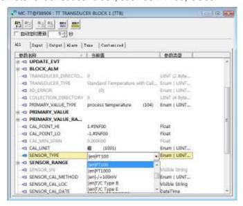
Figure 4.3 Sensor type configuration
