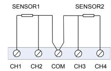
Figure 2.6 Wiring of NCS-TT105 temperature transmitter(3-wire)
