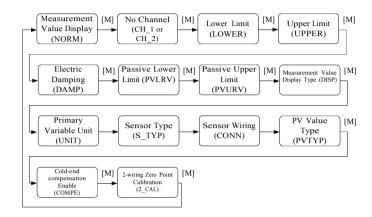
Figure 7.4 Adjusting Function and LCD Display
