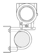
Figure 2.4 The installation of pipe mounting angle bracket-2
