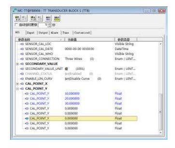
Figure 4.4 CAL\_CURVE\_Y configuration
