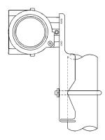
Figure 2.1 The installation of pipe mounting flat bracket
