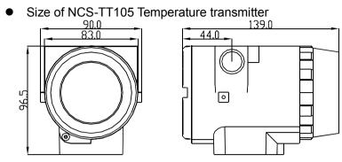
Figure 3.2 Size of NCS-TT105 temperature transmitter (unit: mm)
