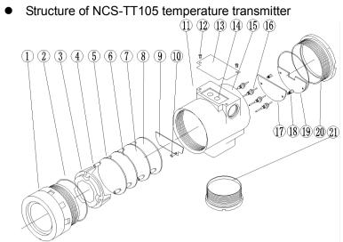
Figure 3.3 Structure of NCS-TT105 temperature transmitter
