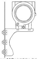
Figure 2.2 The installation of plate mounting angle bracket
