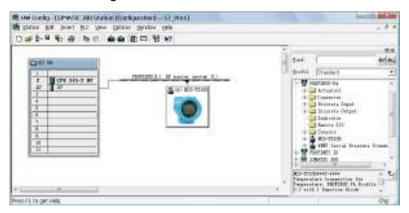
Figure 5.6 Drag it to the PROFIBUS DP bus
