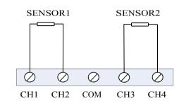
Figure 2.7 Wiring of NCS-TT105 temperature transmitter(2-wire)
