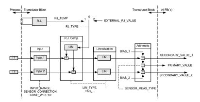
Figure 5.3 Transducer block structure
