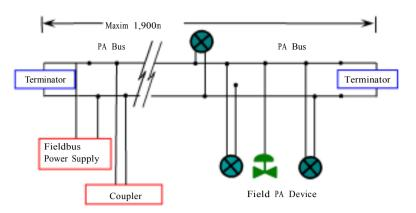
Figure 5.2 PRFIBUS PA bus commection
