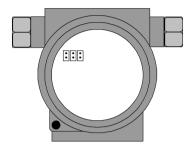
Figure 4.7 NCS-TT105 temperature transmitter hardware jumpers
