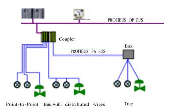
Figure 5.1 PRFIBUS PA network topology
