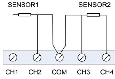
Figure 2.6 Wiring of NCS-TT105 temperature transmitter(3-wire)
