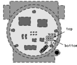
Figure 6.5 HART smart transmitter hardware jumper
