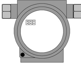
Figure 4.7 NCS-TT105 temperature transmitter hardware jumpers
