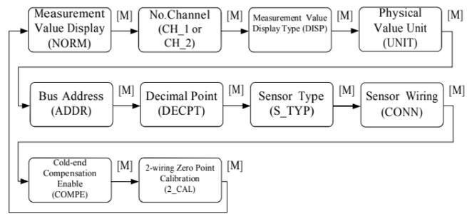
Figure 7.3 Adjusting Function and Display
