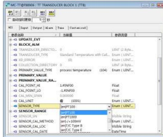
Figure 4.3 Sensor type configuration
