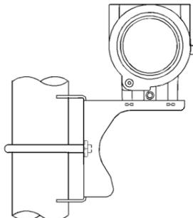
Figure 2.3 The installation of pipe mounting angle bracket-1
