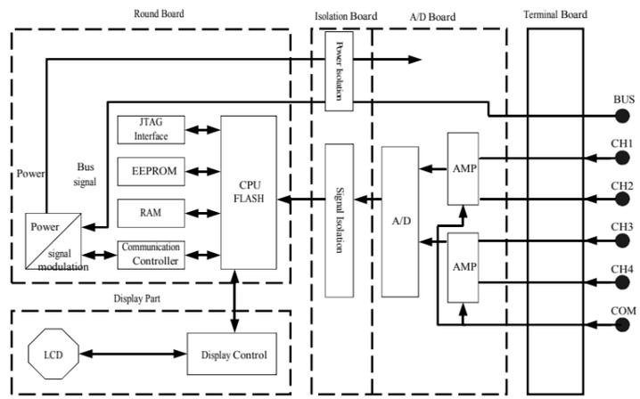
Figure 3.1 Schematic diagram of NCS-TT105 temperature transmitter
