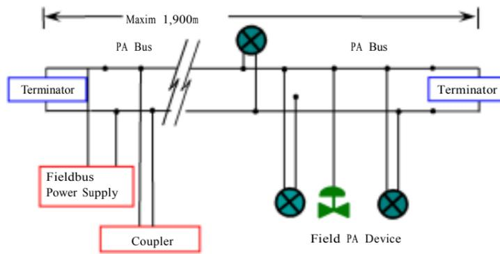
Figure 5.2 PRFIBUS PA bus connection
