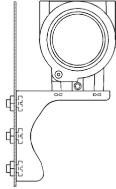
Figure 2.2 The installation of plate mounting angle bracket
