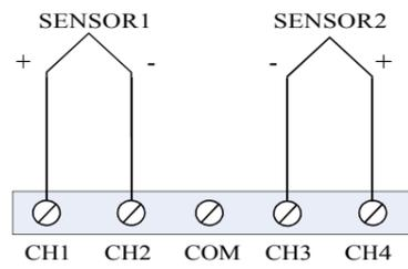
Figure 2.8 Wiring of thermocouple
