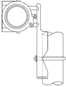
Figure 2.1 The installation of pipe mounting flat bracket
