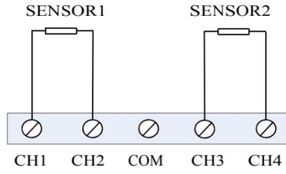
Figure 2.7 Wiring of NCS-TT105 temperature transmitter(2-wire)
