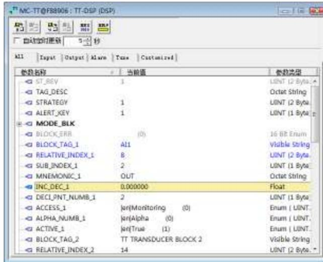
Figure 4.6 Parameter configuration for display block
